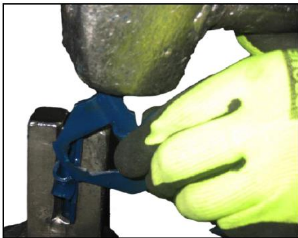
Figure 7: Continue hitting the link, until it clips into the knuckle
