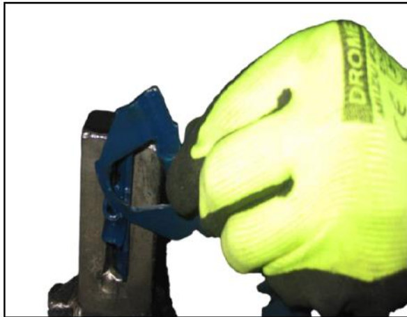
Figure 5: Ensure that it is in the correct position; bring the side of the link as close to the chain breaker as possible in order to get a right (90°) angle.
